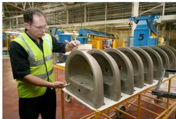
Dimensions change as products go through the different production processes
