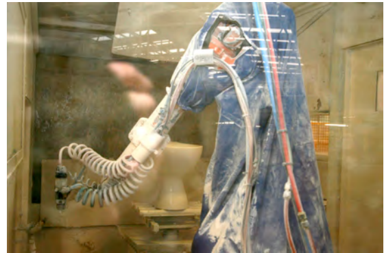
Robot spraying glaze
