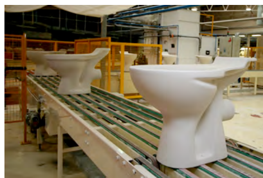
Closets after spraying
